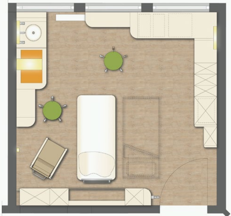
Floor plan drawing of a delivery room, with limited space optimised for the working process. Round-edged built-in furniture underlines fluent movement through space.
